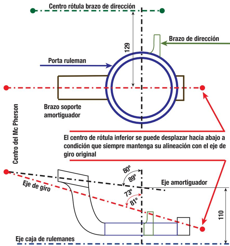
**"A" =  $(80^\circ/89^\circ) \pm 1^\circ$  "B" =  $(73^\circ/81^\circ) \pm 1^\circ$  "C" = 110 mm.  $\pm$  5 mm. "D" = 129mm.  $\pm$  5mm.**
